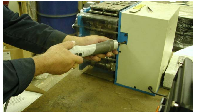
Ingersall Rand Versatec Electric Screwdriver Integrated with a WRC W5-OIB
